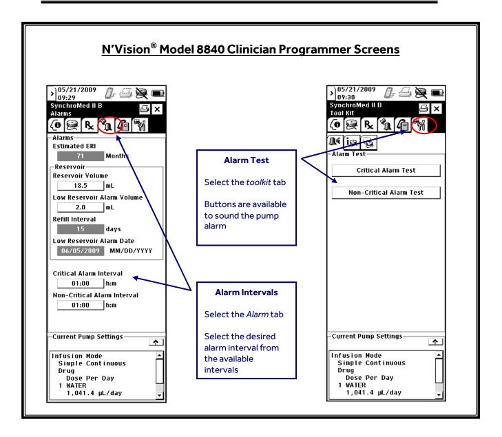
The pump has two different alarms, a **critical** (two tone) alarm and a **non-critical** (single tone) alarm.
